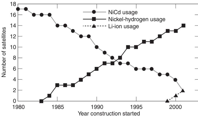
**Figure 1.1.** Noncommercial usage of nickel-cadmium and nickel-hydrogen batteries in satellites during the period when nickel-hydrogen largely replaced nickel-cadmium.
